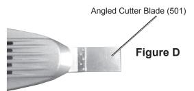
Note: The long Angled Cutter Blade (501) should only be used in the straight ahead position. (See Figure D.)
